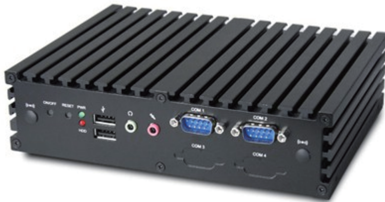
Embedded computer with passive cooling design
